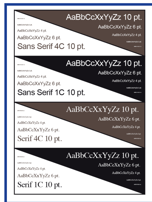
4.1b Minimum Type Size: Using type sizes below a printer's minimum recommended size can result in type filling in.
