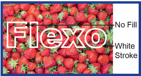
4.1.8b Outline Effect: To create an outline, apply a stroke of the desired color to the type with a fill of none or white. The stroke ought to be at least twice the specified image trap for the applicable print segment.
