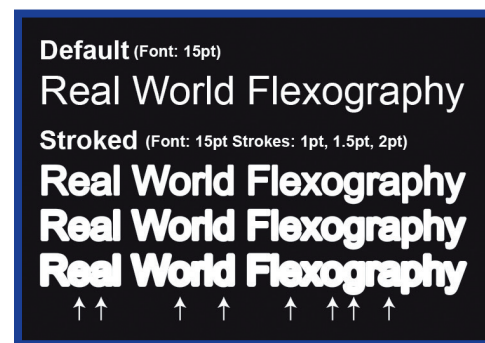
4.1a Typography: As copy is stroked or bolded the counters (holes in letters such as a, d, o, e and R) may begin to fill in during print.
