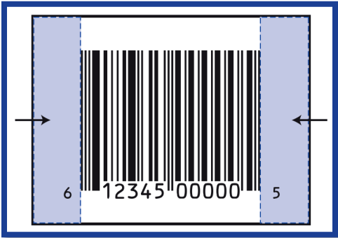
4.3.2d Quiet Zones: Quiet zones allow scanners to detect when a bar code starts and stops. Minimum quiet zone specifications depend on the code and its magnification.
